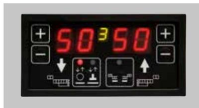
FOX 500 KRT. This control unit synchronises the lowering and raising of the platen to any feed speed rating of the conveyor.
